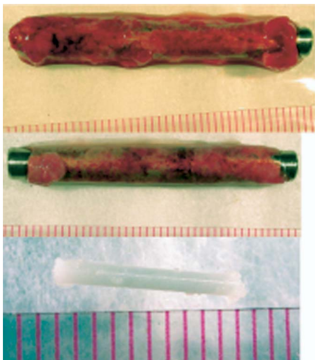
Figure 4 Rocker test system results of thrombus formation being conducted to assess material compatibility. The top two panels show the industry standard Ti Alloys covered with thrombus after rocker test. The bottom panel shows YTZP Zirconia Ceramic with little deposition after the same test.
